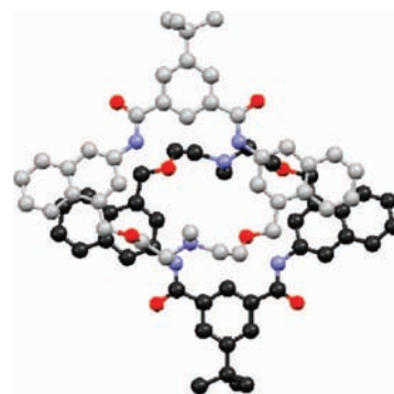
Figure 1. X-ray crystal structure of the macrocycle 3 ; the unit cell packs as a cofacial dimer.
